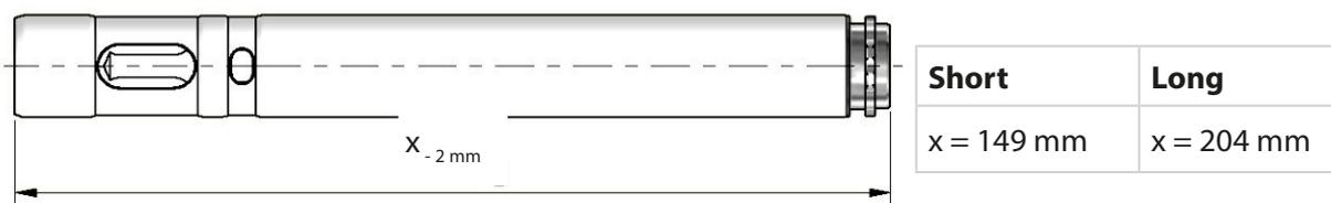
High process pressures and high process temperatures can cause the immersion tube to shrink (known creep tendency of PTFE).
