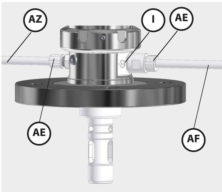
1. Connect the outlet hose (**AF**) using the hose coupling (**AE**). The outlet is marked with the following symbol (**I**).
