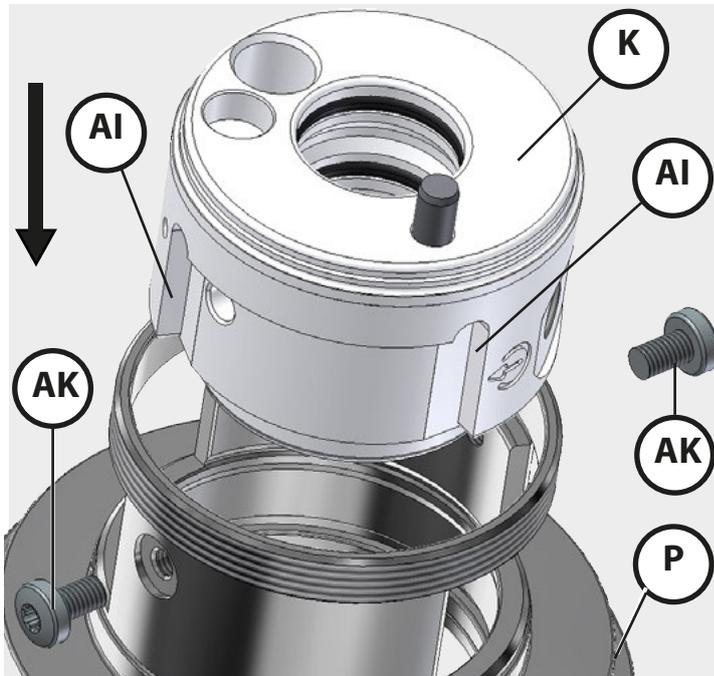
1. Align the guiding edges (**AI**) of the calibration chamber (**K**) and insert it in the process adaptation (**P**).
