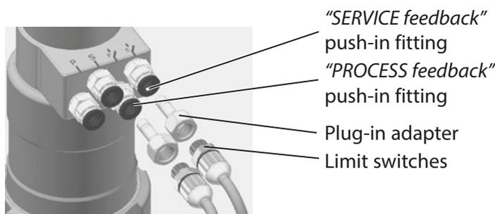
1. Screw the plug-in adapters onto the limit switches.
