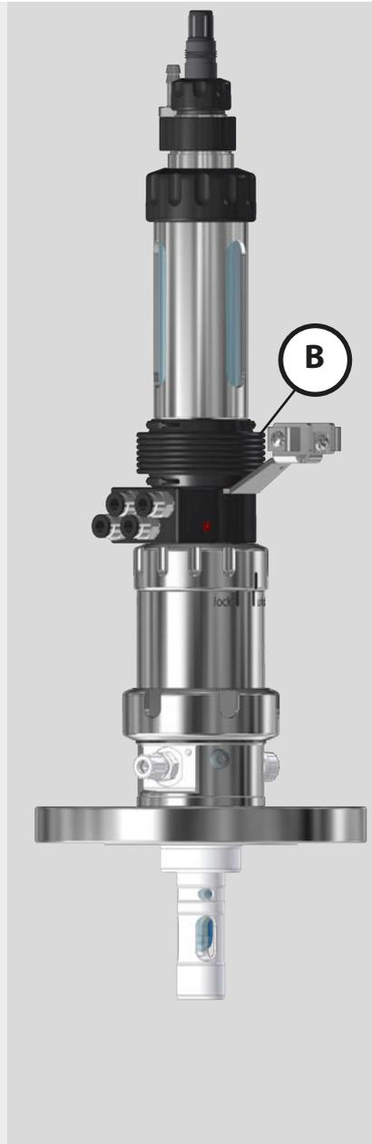
The PROCESS position is indicated by the rubber bellows (**B**) being compressed.
