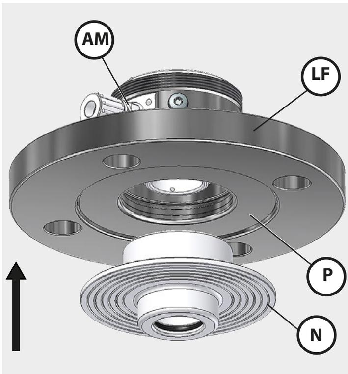
3. Install the loose flange (**LF**) if required. Screw in the inlet and outlet (**AM**) connectors.
