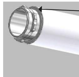
Stop for the screws on the immersion tube
