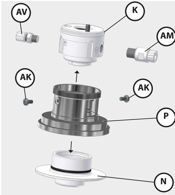
1. Screw off the outlet (**AM**) and inlet connectors (**AV**). Take off the loose flange if required.
