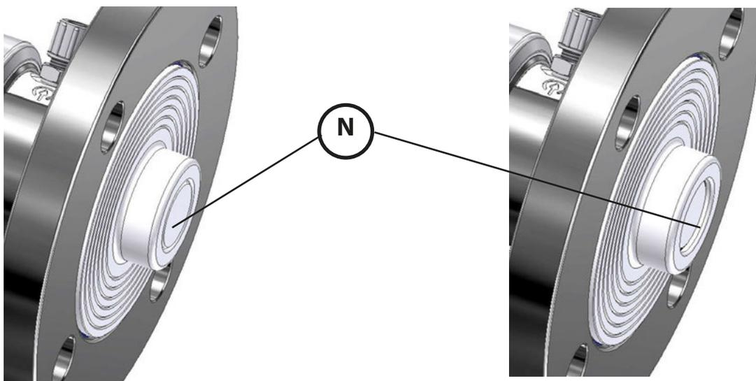
As delivered, the immersion tube fits flush with the flange bushing (N).
