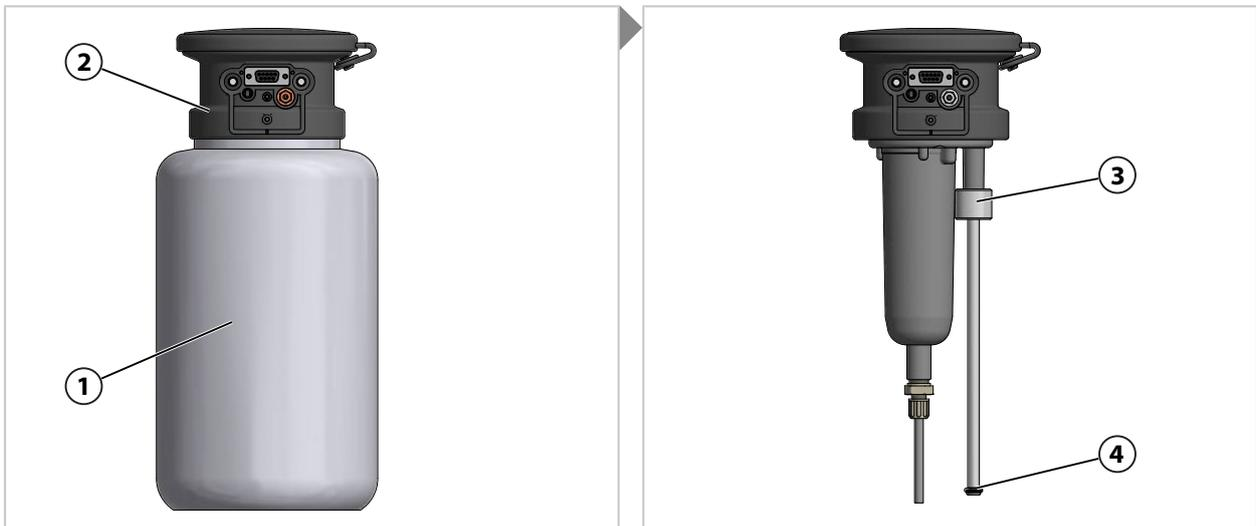
03. Unscrew the container **(1)** from the pump head **(2)**.
