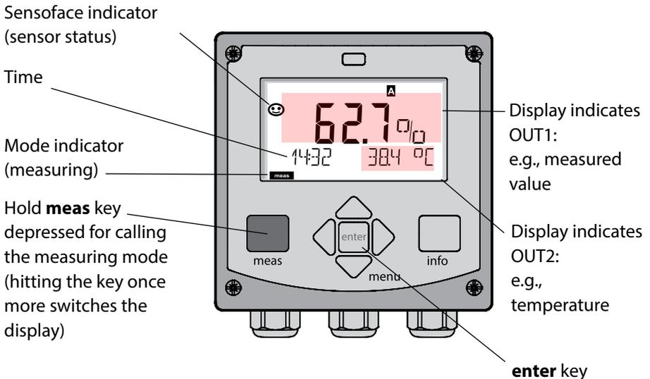
Depending on the configuration, you can set various displays as standard display for the measuring mode (see page 20).
