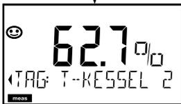
By pressing **meas** briefly you can step through further displays such as primary value or tag number (TAG). After 60 sec they switch back to the main display.
