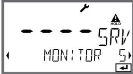
**Displaying currently measured values (sensor monitor) with HOLD mode activated:**
