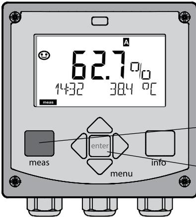
The MAIN DISPLAY is the display which is shown in measuring mode. To call the measuring mode from any other mode, hold the **meas** key depressed for at least 2 sec.
