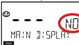
Press **enter** to select a display as MAIN DISPLAY (displayed permanently in measuring mode).
