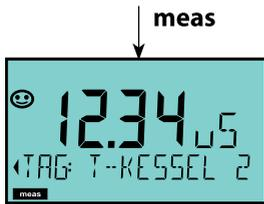
By pressing **meas** briefly you can step through further displays such as tag number (TAG) or flow (L/h).
