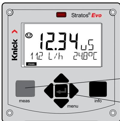
The MAIN DISPLAY is the display which is shown in measuring mode. To call the measuring mode from any other mode, hold the **meas** key depressed for at least 2 sec.
