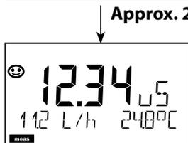
By pressing **meas** briefly you can step through further displays such as tag number (TAG) or flow (L/h).
