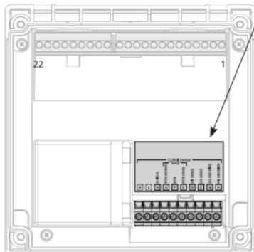
The measuring module comes with a self-adhesive label. Stick the label to the module slot on the device front. This way, you have the wiring "under control".
