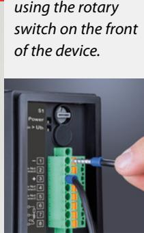
Quick, safe wiring of output and power supply using push-in spring-cage terminals
