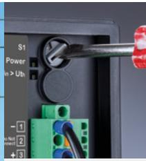
10 default threshold values can be selected using the rotary switch on the front of the device.
