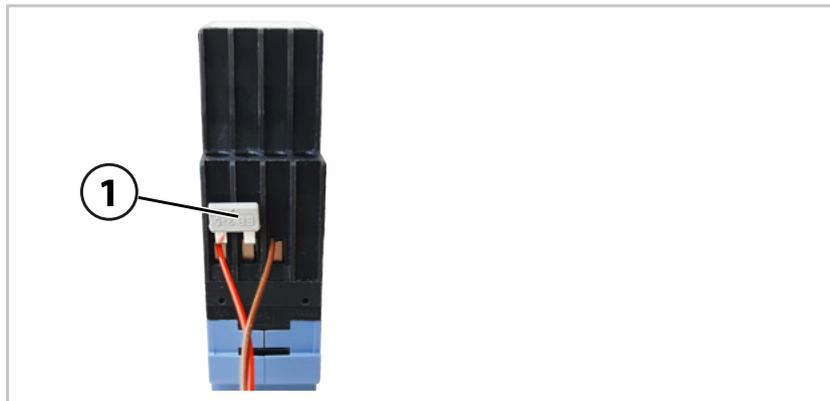
10. Connect the cables for the input. Mount the insertable jumper (**1**) according to the desired input range (see example figure: Insertable jumper in terminals 5 and 6).
