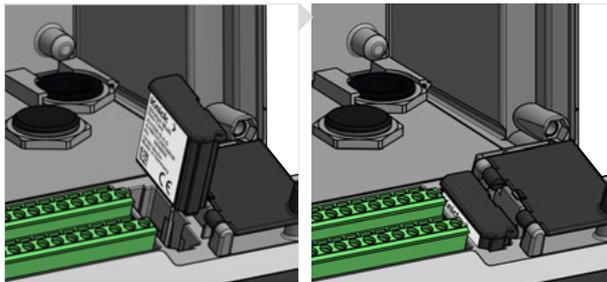
06. Close the enclosure and successively tighten the enclosure screws in a diagonal pattern.
