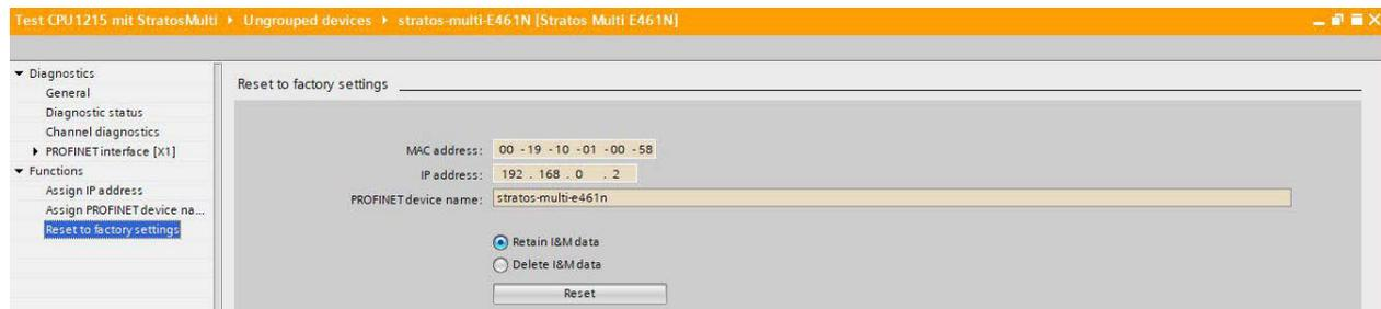
The reset function via PROFINET does not reset the Stratos Multi to its factory settings.
