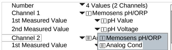
Assign a sensor to the second channel.
