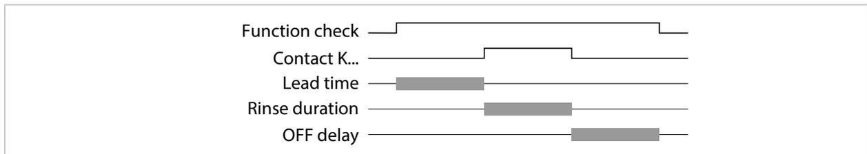
**Note:** Function Check (HOLD) is activated from the start of the lead time until the end of the OFF delay. The current outputs and remaining relay contacts behave in accordance with the parameter settings.
