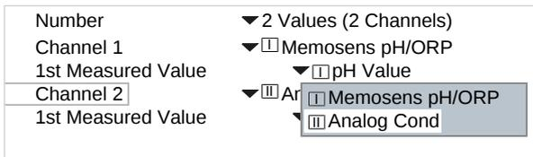
Assign a sensor to the second channel.
