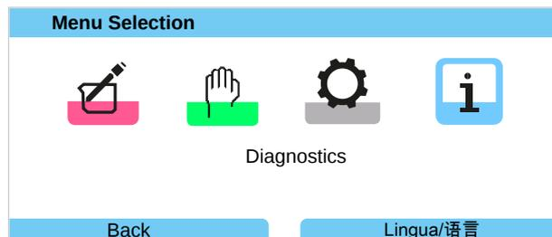
Diagnostic functions can be directly opened from the measuring mode with the **right softkey**. To do this, the Favorites menu function must be assigned to the **Softkey (1)**:
