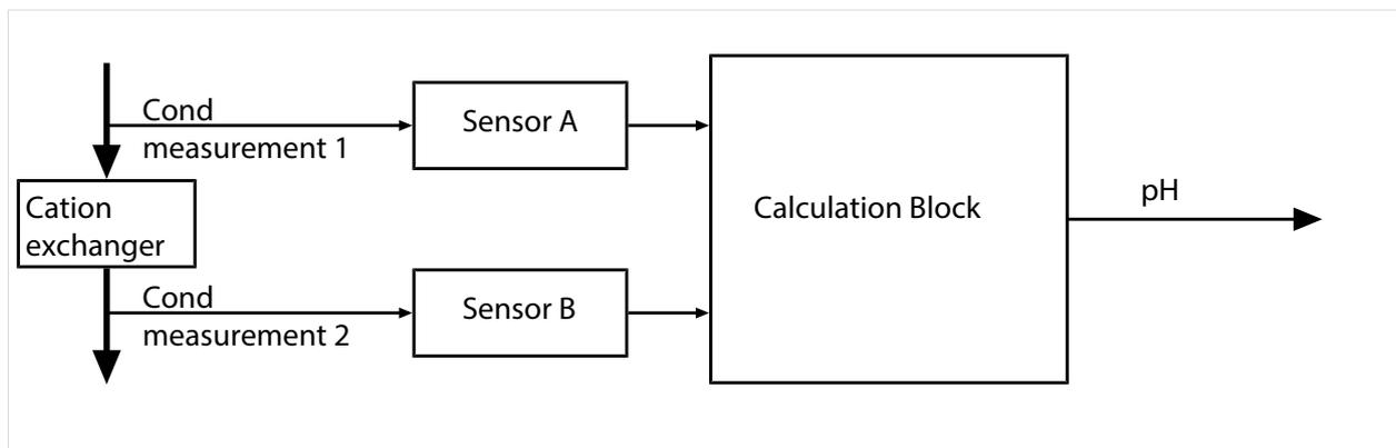
**Calculating the concentration of caustic soda solution/the pH value:**
