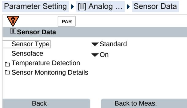
01. In **Temperature Detection**, select the used temperature probe and whether the temperature is to be measured automatically or manually during measurement and/or calibration.
