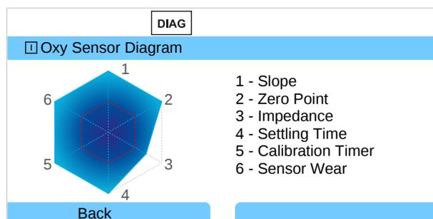
The tolerance limits (radius of the “inner circle”) can be changed as required:
