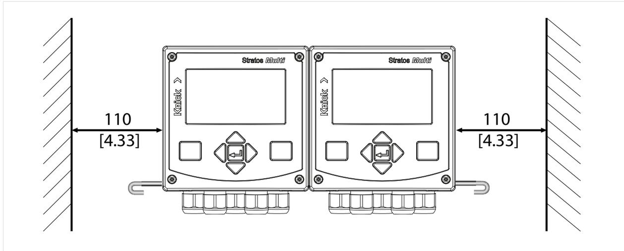
There is a 100 mm hinge pin in the bag containing small accessory parts included in the package contents → *Package Contents and Product Identification*, p. 12. The hinge pin connects the front and rear units. Depending on space requirements, the hinge pin can be inserted on the left or right. In order to replace the front unit, a minimum clearance of 110 mm [4.33 inches] must be maintained on the relevant side.
