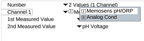
Assign a sensor to the channel.
