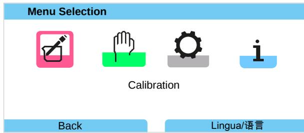
**Note:** During calibration, the function check mode (HOLD) is active for each of the calibrated measuring channels. The outputs respond as configured.
