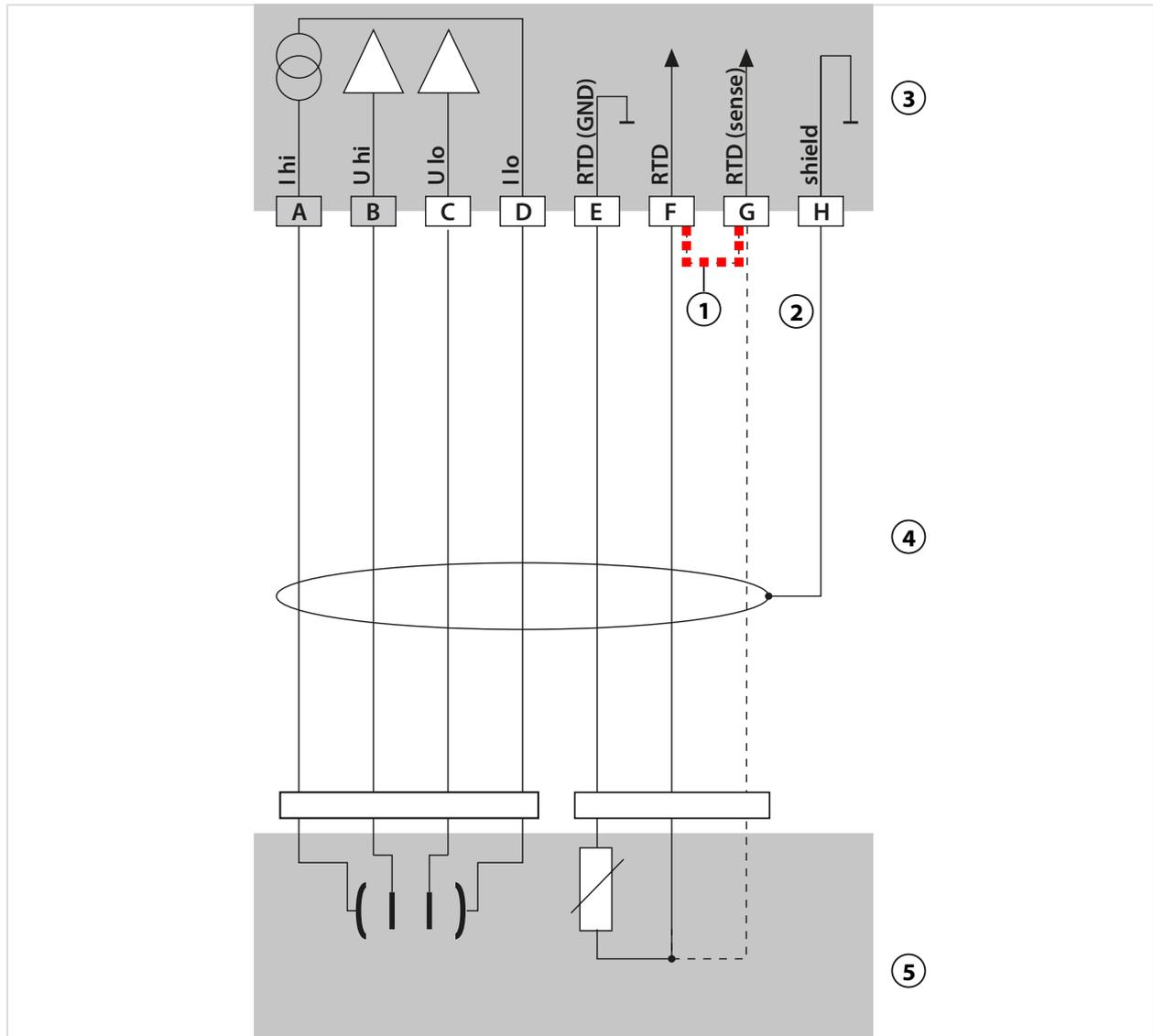
1 Set jumper between F and G if a 2-wire temperature detector is used!
