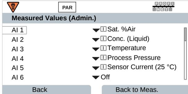
The measured values available are determined by the connected sensor and the configuration.
