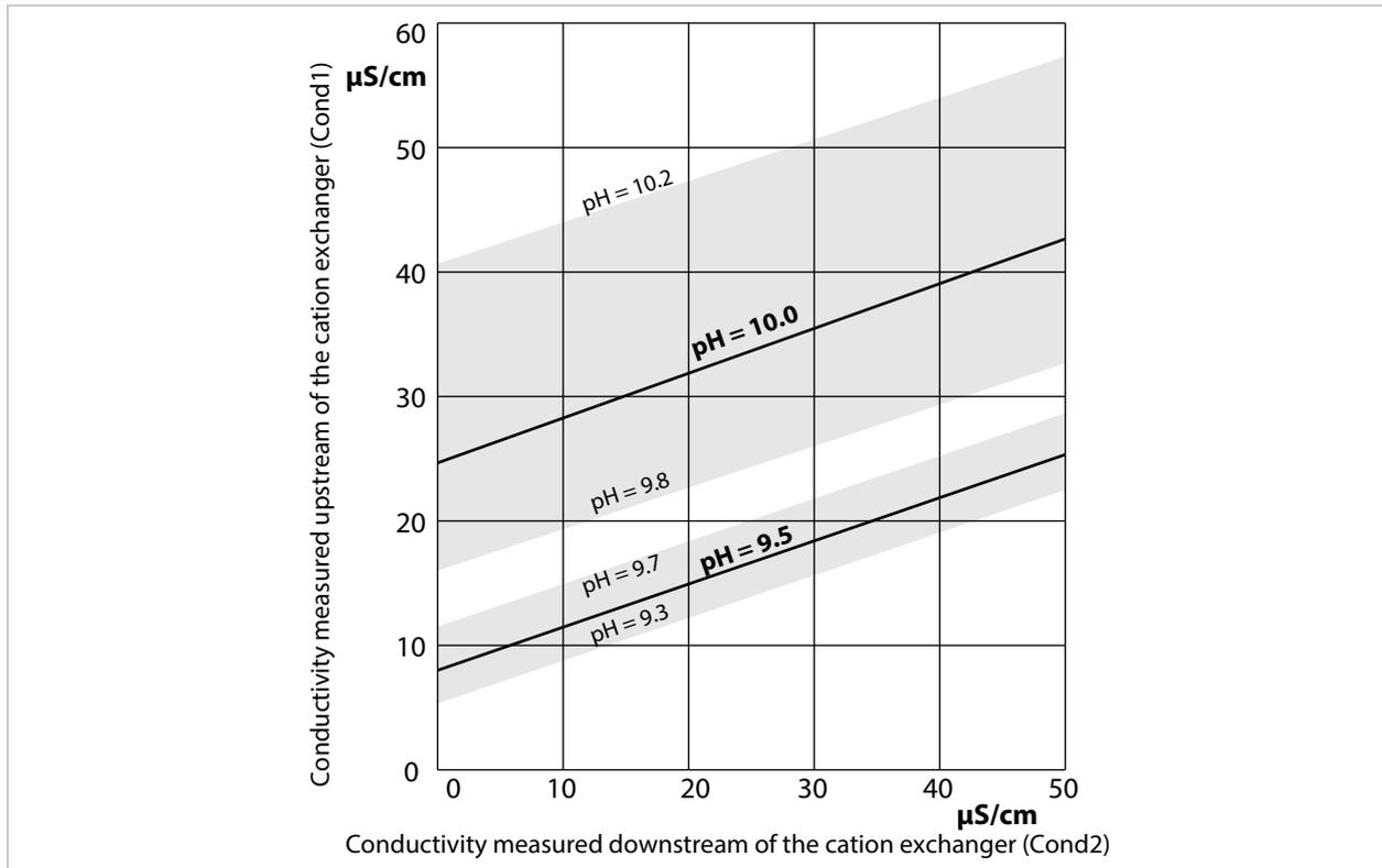
Conditioning the boiler water in natural circulation boilers with sodium hydroxide. Relationship between the pH value and the conductivity measured upstream or downstream of the cation exchanger.
