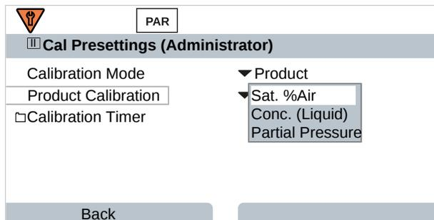
The settings are made in the Cal Presettings submenu:
