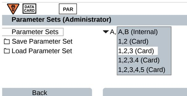
**Note:** As soon as parameter sets are selected on the Data Card, OK2 “Parameter Set Selection” is set to “Off”.
