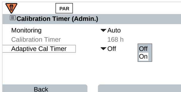
**Note:** If Sensoface is enabled, a neutral smiley is displayed once 80 % of the interval has expired. Once the entire interval has expired, a sad smiley is shown, a Maintenance Required message is generated, and the corresponding NAMUR icon is displayed and the measurement display is shown with blue backlighting (display color: NE107). If the current outputs have the correct parameter setting, a 22 mA error signal is generated.
