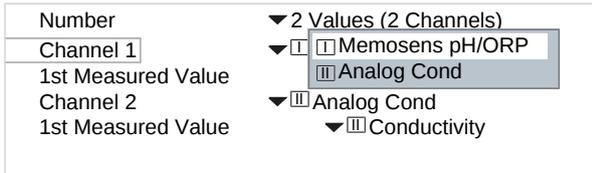
Assign a sensor to the first channel.
