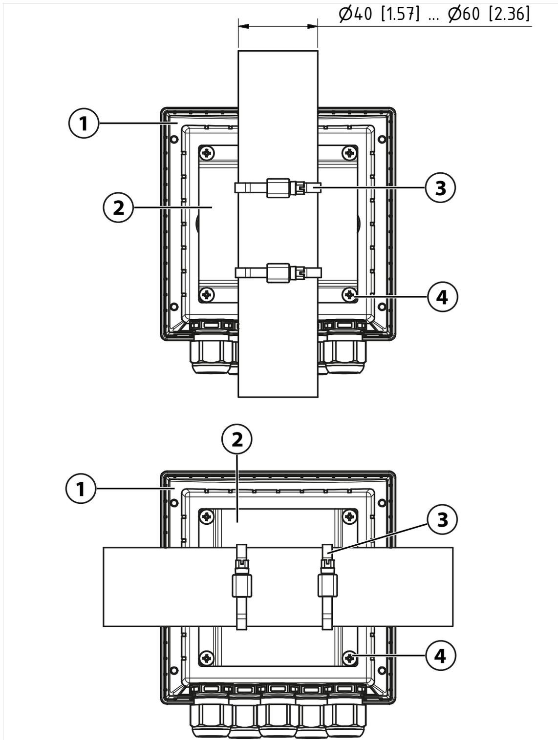
1 For either vertical or horizontal posts or pipes
