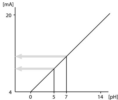
Example measuring span pH 5 ... 7
