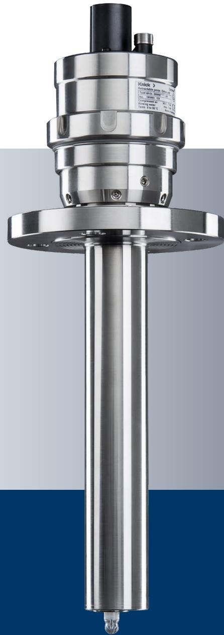
Flexible immersion fitting; customer-specific immersion depths from 150 mm to 275 mm. This retractable fitting is dimensioned for operation with electrochemical sensors (Ø 12 mm) with a length of 425 mm or 450 mm for pressurizable sensors or optical sensors (Ø 12.7 mm).
